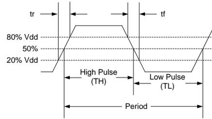
Figure 3. Output Waveform
