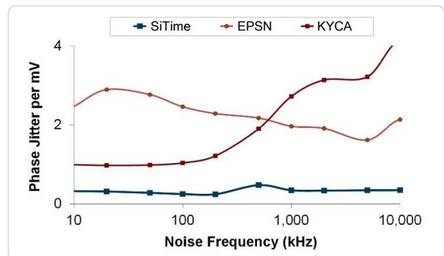
Figure 4. Power Supply Noise Rejection<sup>[4]</sup>
