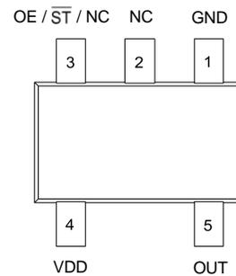
**Figure 1. Pin Assignments**
