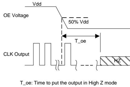
T\_oe: Time to put the output in High Z mode
