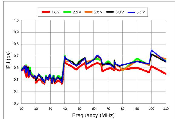
Figure 15. RMS Integrated Phase Jitter Random (900 kHz to 20 MHz) vs Frequency<sup>[9]</sup>
