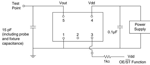
Figure 2. Test Circuit
