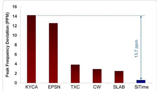
Figure 6. Shock Robustness<sup>[6]</sup>
