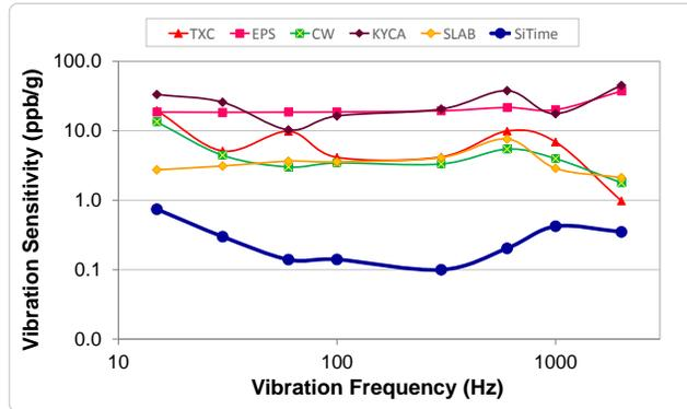
Figure 5. Vibration Robustness<sup>[5]</sup>
