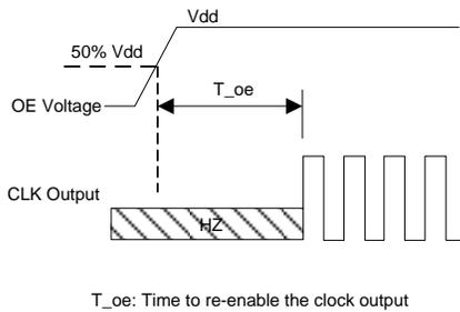
T\_oe: Time to re-enable the clock output
