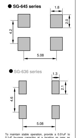
To maintain stable operation, provide a 0.01uF to 0.1uF by-pass capacitor at a location as near as possible to the power source terminal of the crystal product (between Vcc - GND).
